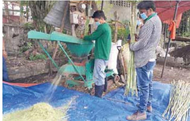
*Workers demonstrate the milling process of decorticated Napier stalk*
