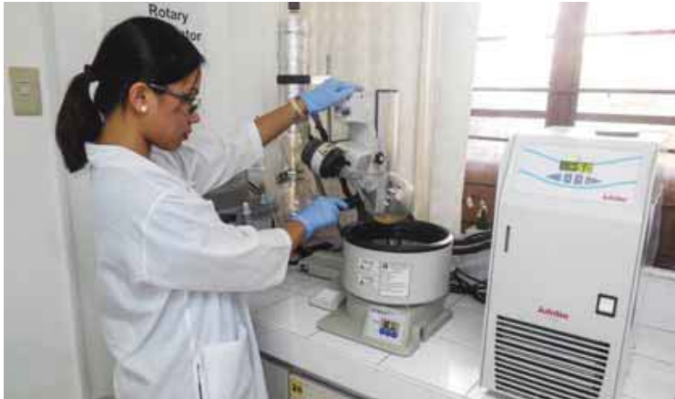
Concentration of honey samples in vacuo by rotary evaporation at 40°C
