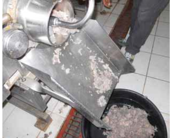
Mincing of fish using meat and bone separator. During this process, the muscle is separated from the bones and skin
