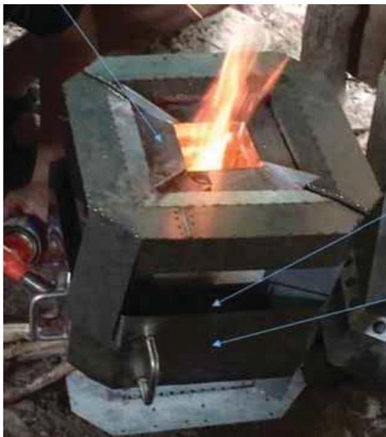
*Bathala Version 2 prototype, a rocketstove that simultaneously cooks food using less fuel, generates electricity, and distills or boils water for drinking*
